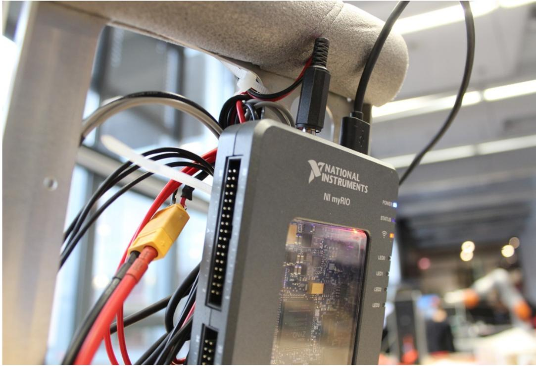
Figure 5. Single NI myRIO USB communication controlling all servo motors.
