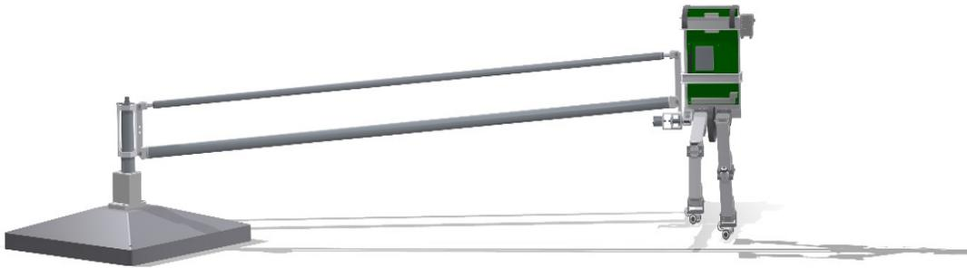
Figure 1. Leo – the bipedal humanoid robot laterally stabilized by a boom and performing circle walking.
