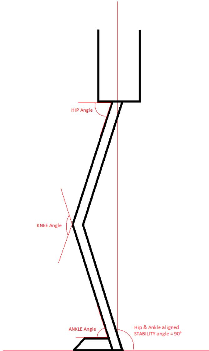
Figure 3. Ankle, knee and hip angles involved in the mathematical model and controller.
