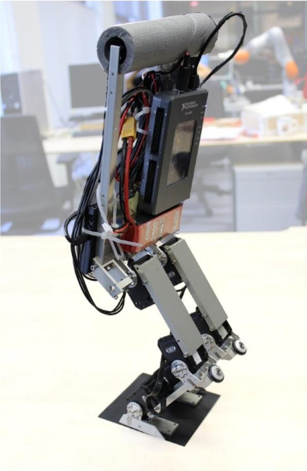
Figure 2. Stand-alone bipedal humanoid robot performing squats using NI myRIO.
