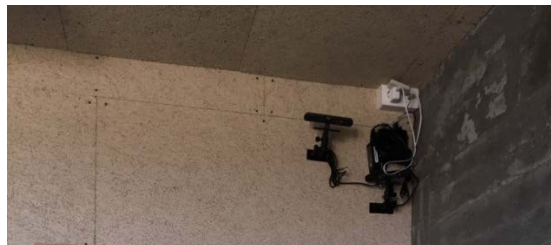
Picture 4: Detail of the Pentalo 3D cameras and KIO beacons for motion capture
